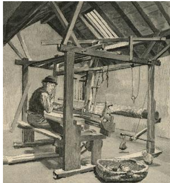
Weaver at work on a typical loom of the 18 th century – Perthshire, Crieff and Strathearn Local History Society
